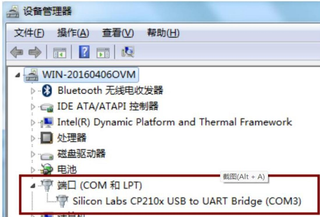
Open "Port" to view the port number as shown in the figure, "Silicon Labs CP210× USB to UART
